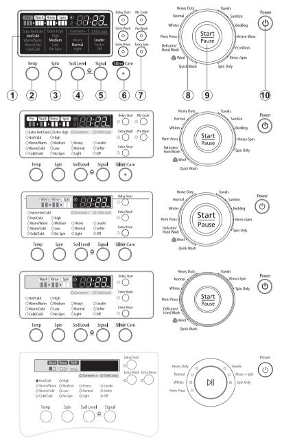
Digital graphic display Displays the remaining cycle time, all cycle information, and error messages.
