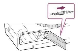
Insert the battery pack while pressing the lock lever (A) with the tip of the battery until the battery locks into place.
