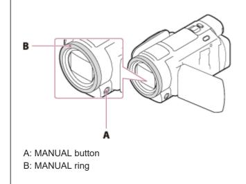
Rotate the MANUAL ring to make adjustments.
