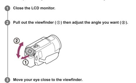
If the indicators on the viewfinder appear blurred, adjust it using the viewfinder lens adjustment dial located on the side of the viewfinder.
