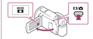
Press PHOTO lightly to adjust the focus, then press it fully.
