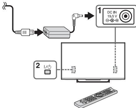
**1** Complete your cable connections before proceeding with the **Initial Setup**. Connect the AC power cord to the AC adapter and plug the AC adapter to the TV in the DC IN 19.5 V terminal. Then, connect the AC adapter to your nearest power outlet.
