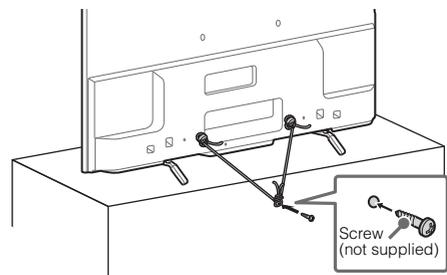
The length of the M6 machine screw differs depending on the rope or chain diameter. Please see below illustration.
