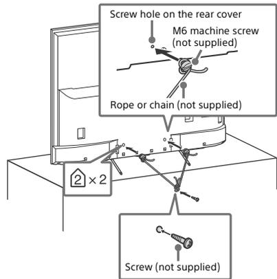
The length of the M6 machine screw differs depending on the rope or chain diameter. Please see below illustration.
