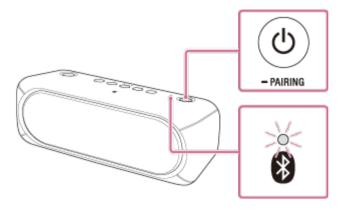
When you turn on the speaker, the speaker tries to make a BLUETOOTH connection with the last connected BLUETOOTH device. If the device is nearby and its BLUETOOTH function is on, the BLUETOOTH connection is established automatically and the **(BLUETOOTH)** indicator stays lit. When you want to connect another BLUETOOTH device, terminate the current BLUETOOTH connection by operating the currently connected BLUETOOTH device.
