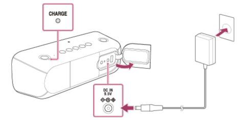
Charging starts and the CHARGE indicator lights up in orange. Charging is completed in about 4 hours<sup>\*1</sup> and the indicator turns off. Once the battery is fully charged, it will not be charged further even if the speaker is kept connected to an AC outlet.
