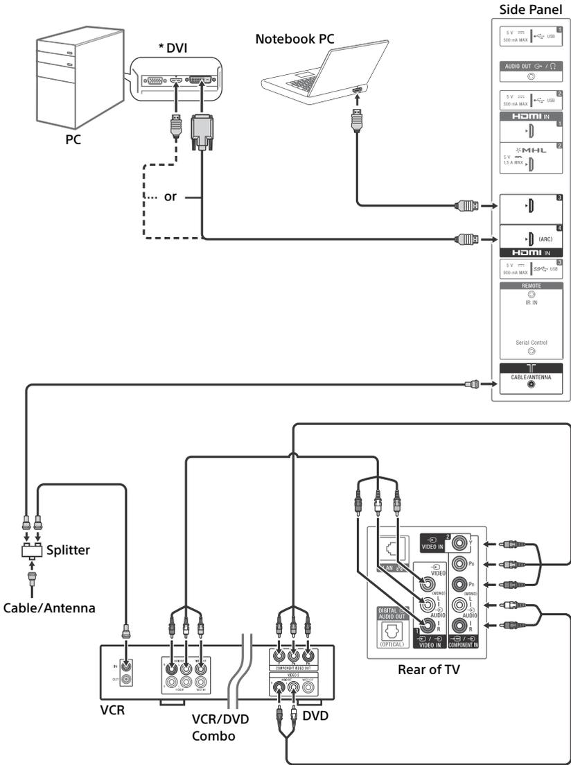
\* DVI does not support audio signals. Connect the audio output of the PC to the PC speakers or an A/V receiver to listen to sound from the PC.
