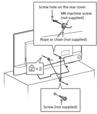
The length of the M6 machine screw differs depending on the rope or chain diameter. Please see below illustration.
