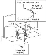
The length of the M6 eye bolt differs depending on the rope or chain diameter. Please see below illustration.
