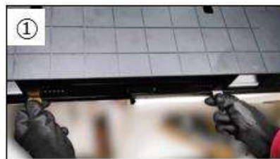
Locate both hooks and unhook using coin/Jig.
