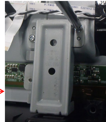
Remove the BOTTOM FRAME
