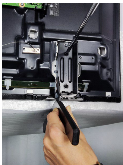
3. Hold the Stand while unscrewing
