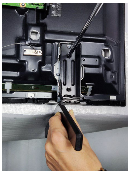
3. Hold the Stand while unscrewing
