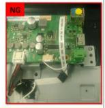
Make sure Connector Assy 10P wire not wrap around FFC 5P
