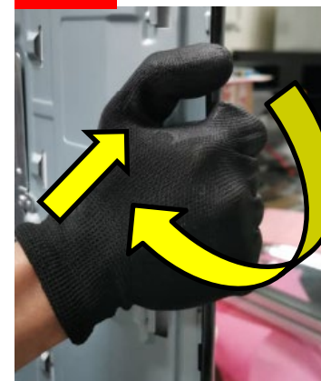
Since the O-cell may pop out, DO NOT apply force to the Back Chassis or rotate the Bezel
