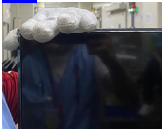
Holding edge of the Bezel without touching the O-cell
