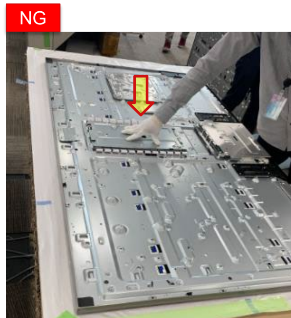
Press on P-mod during Assy & Disassy
