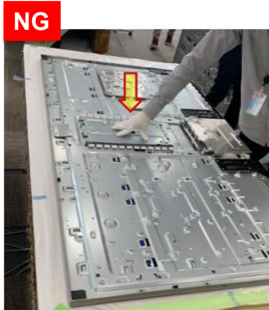
Press on P-mod during Assy & Disassy
