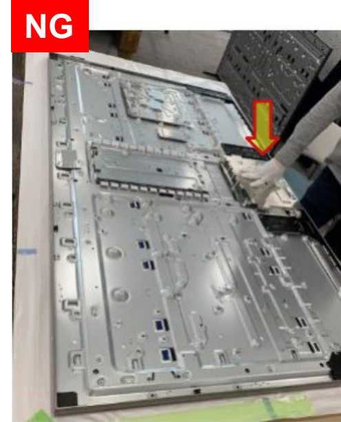
Press on P-mod during Assy & Disassy
