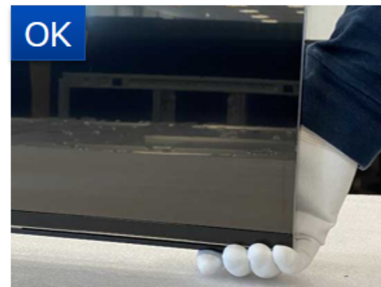
Support set at edge of BZ without touching o-cell
