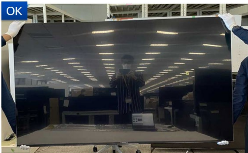
Carry P-mod by vertical position
