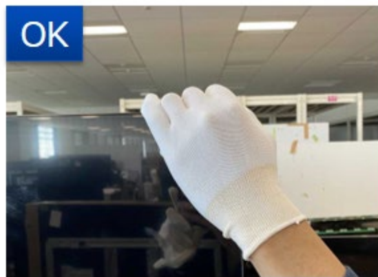
Holding edge of BZ without touching o-cell
