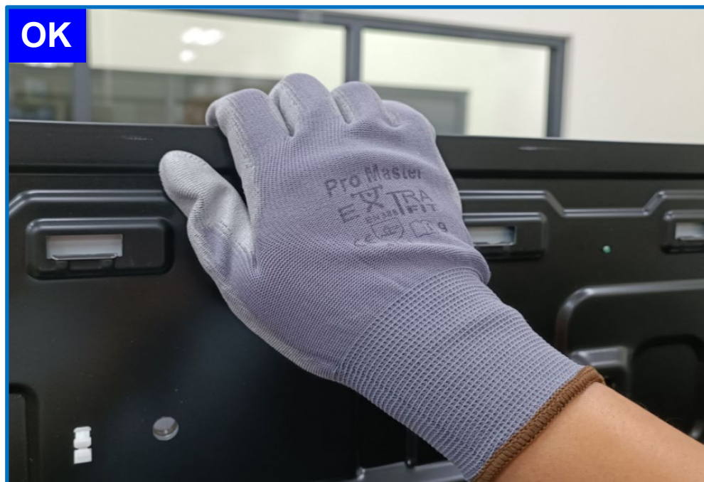
Avoid touch Rear Cover hook during P-mod handling
