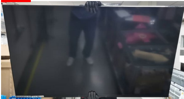
DO NOT carry the panel at the center area
