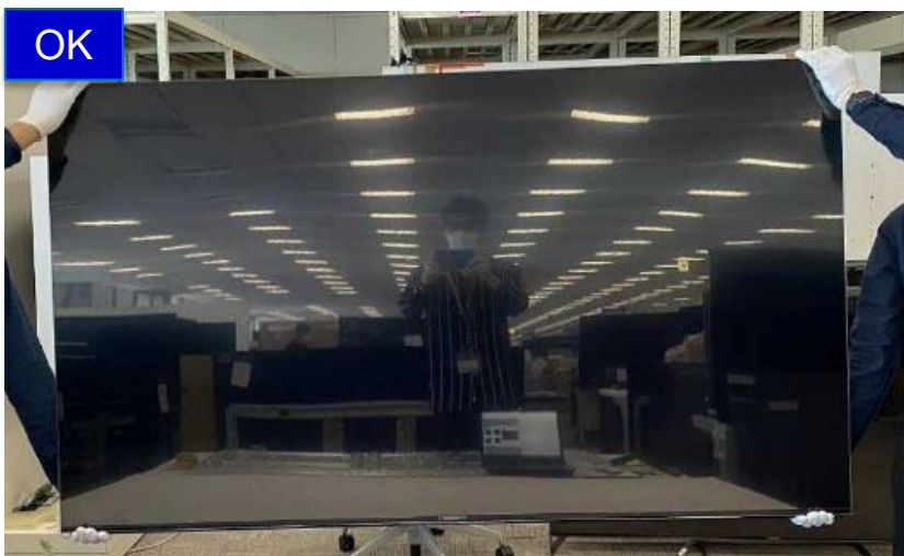
Carry P-mod by vertical position
