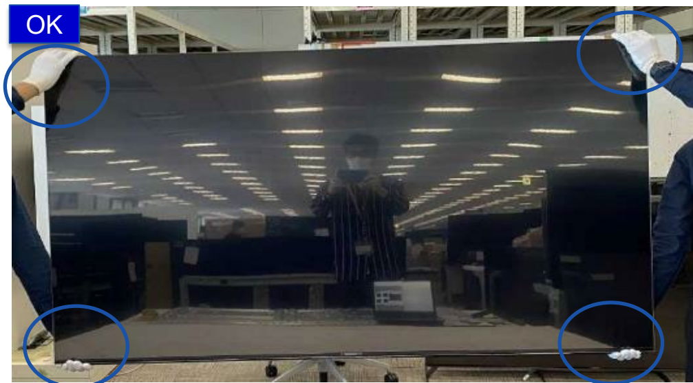
Always wear gloves during P-mod handling
