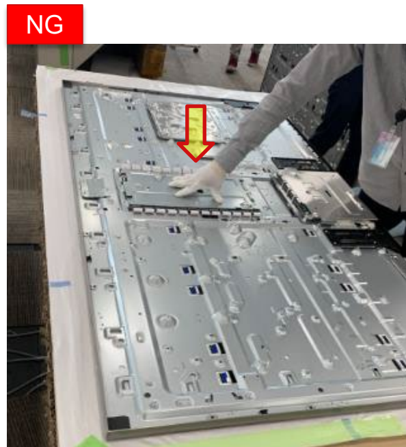
Press on P-mod during Assy & Disassy
