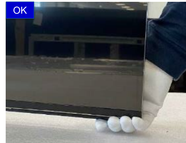
Support set at edge of Bezel without touching O-cell
