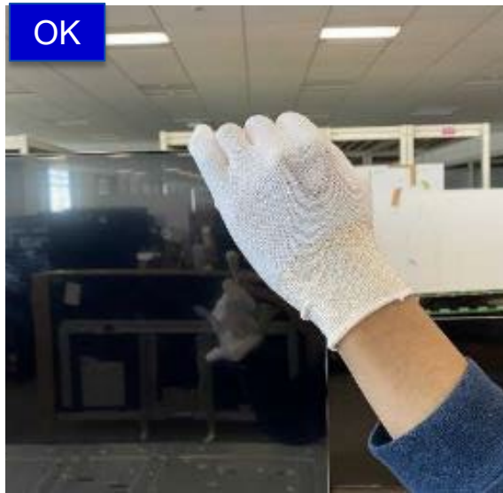
Holding edge of Bezel without touching O-cell
