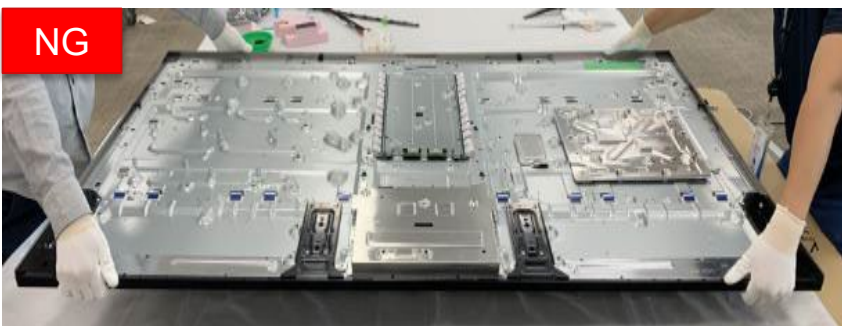
Carry P-mod by horizontal position
