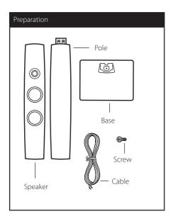
1. Attach the pole to the base, then secure the connection with a supplied screw.
