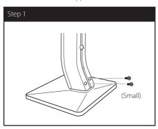
2. Secure the connection with a supplied screw, then insert a speaker wire from the bottom of the base.
