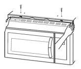
4. Remove the cover screw,pull the cover forward and then lift up the bulb holder.
