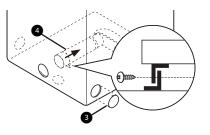
3 Preassemble a 4" (10 cm) elbow S to the next 4" (10 cm) duct section, and secure all joints with duct tape. Be sure that the male end of the elbow faces AWAY from the dryer. Insert the elbow/duct assembly through the side opening and press it onto the adapter duct. Secure it in place with duct tape. Be sure that the male end of the duct protrudes 1 1/2" (3.8 cm) to connect the remaining ductwork. Attach the cover plate S to the back of the dryer with the included screw.
