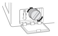
**8** Close the drain pump filter cover.
