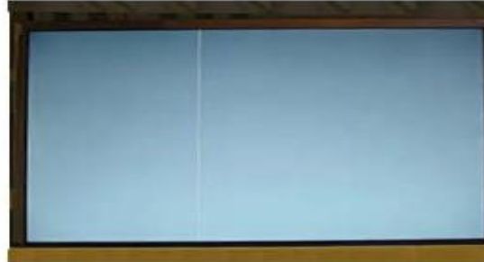
Vertical Line Source TAB IC Defect
