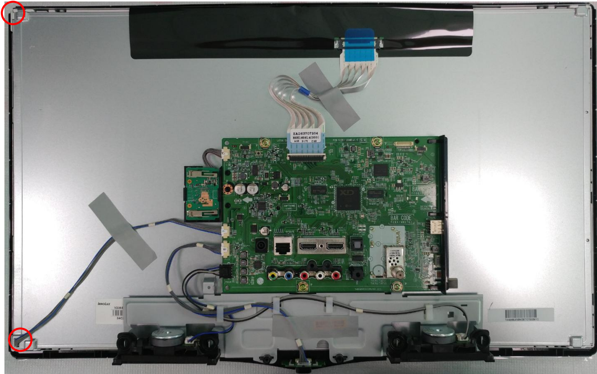
Power On -> disjoint back case -> check lighting
