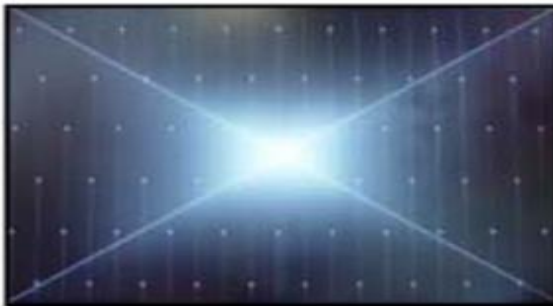
Solder defect, Short/Crack
