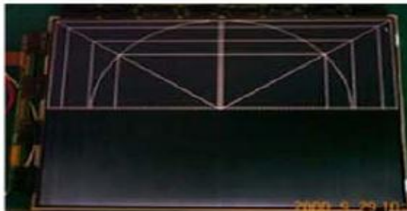
Horizontal Block Gate TAB IC Defect
