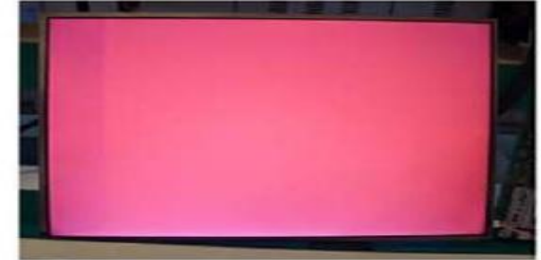
Vertical Block Source TAB IC Defect
