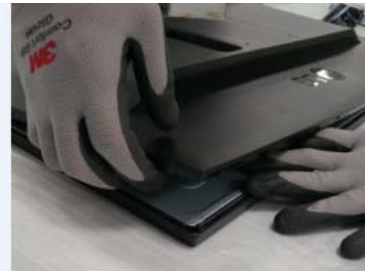
1.The open status top/side of both , one hand was supported module, and open the Back cover.
