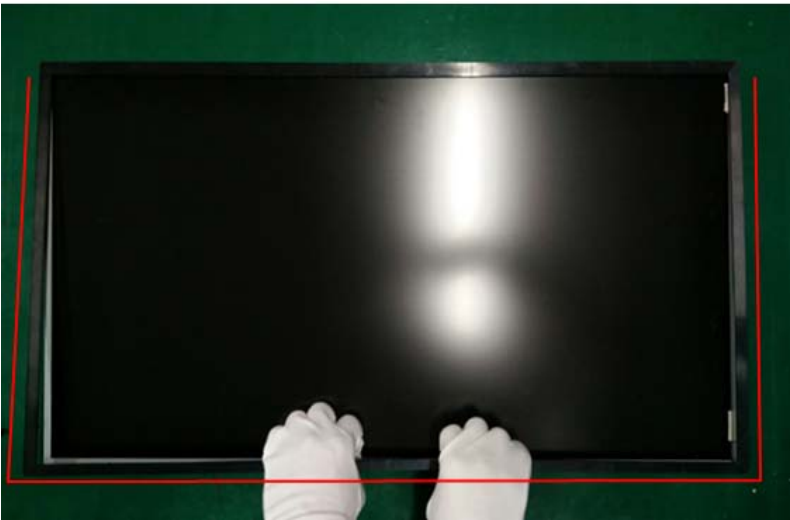
○ Fig 4 overturn the set and disassemble the latches of three edges.
