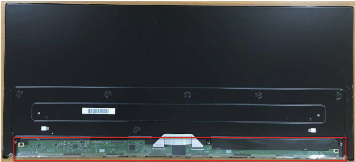
Fig 9 Remove T-con sheet
