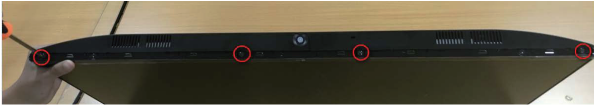
Fig 5 Remove bottom screw(4EA)
