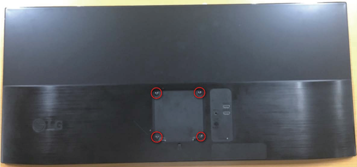
Fig. 3 Remove the Screw(4EA)
