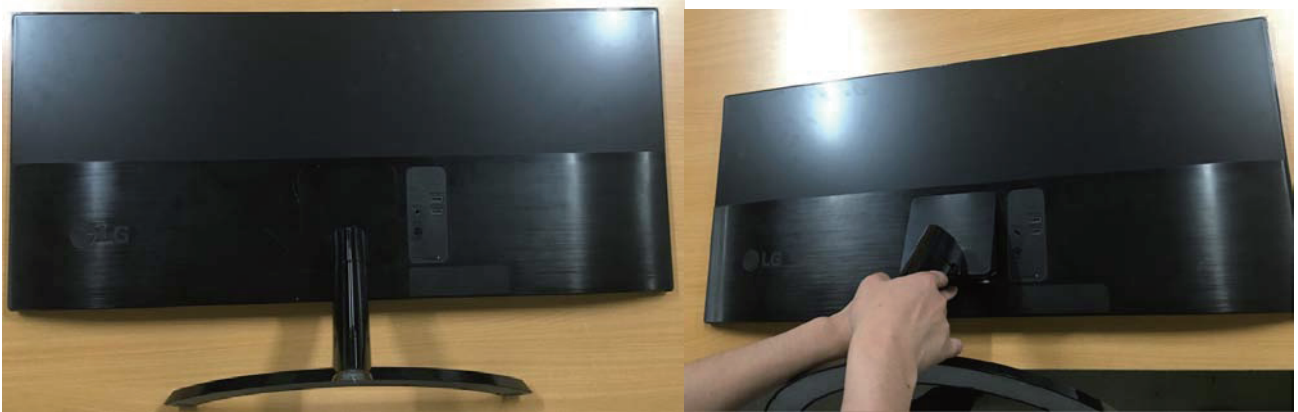
Fig.1、 2 Put the MNT on the clean and flat surface, disassembly the stand assy(press down joy button)
