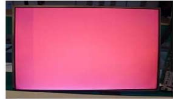
Vertical Block Source TAB IC Defect
