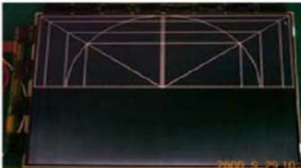
Horizontal Block Gate TAB IC Defect
