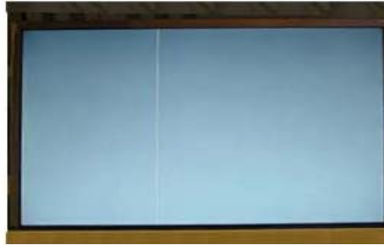
Vertical Line Source TAB IC Defect
