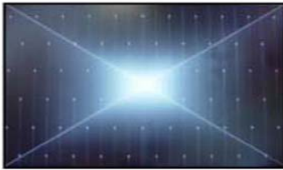
Solder defect, Short/Crack
