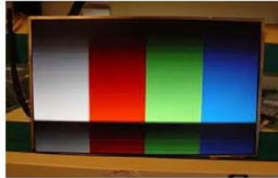
Horizontal Block Gate TAB IC Defect
