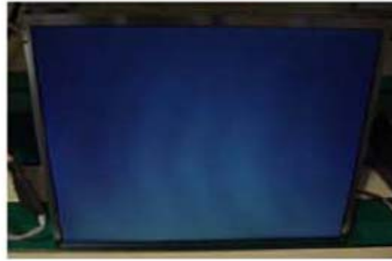
Panel Mura, Light leakage
