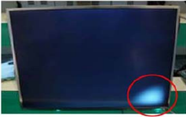
Panel Mura, Light leakage
