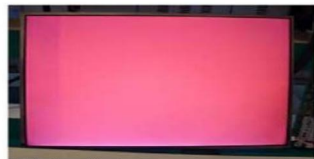
Vertical Block Source TAB IC Defect
