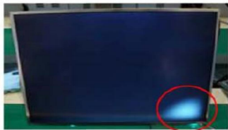
Panel Mura, Light leakage
