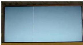
Vertical Line Source TAB IC Defect
