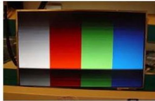
Horizontal Block Gate TAB IC Defect
