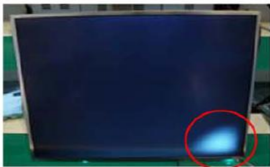
Panel Mura, Light leakage
