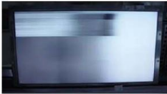
Horizontal Block Gate TAB IC Defect
