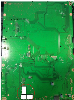
Tuner GND is separated.
