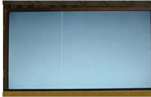
Vertical Line Source TAB IC Defect
