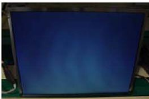
Panel Mura, Light leakage
