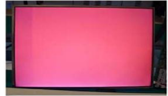
Vertical Block Source TAB IC Defect
