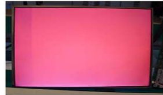
Vertical Block Source TAB IC Defect
