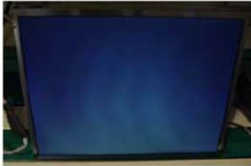
Panel Mura, Light leakage
