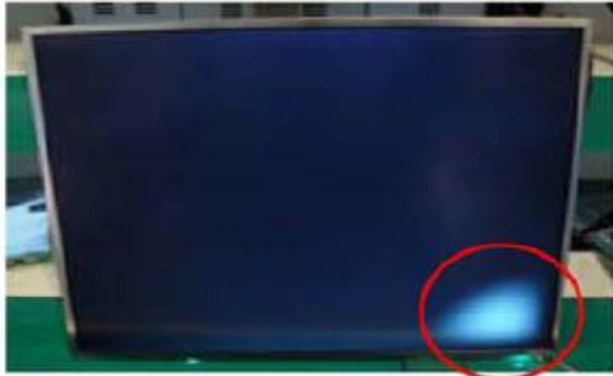
Panel Mura, Light leakage
