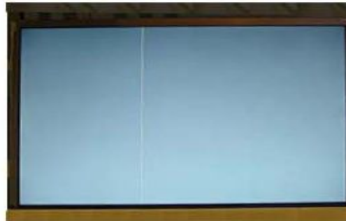
Vertical Line Source TAB IC Defect
