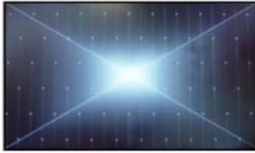
Solder defect, Short/Crack
