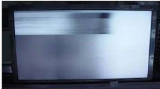
Horizontal Block Gate TAB IC Defect
