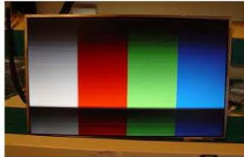
Horizontal Block Gate TAB IC Defect
