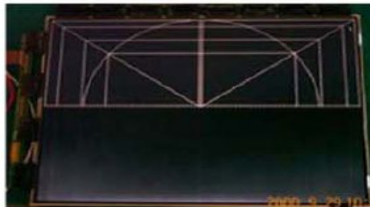
Horizontal Block Gate TAB IC Defect
