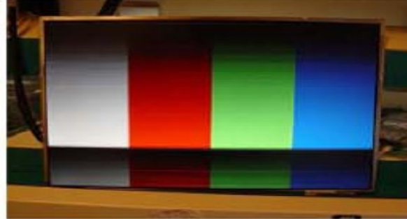
Horizontal Block Gate TAB IC Defect
