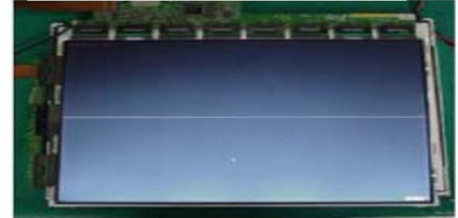
Horizontal line Gate TAB IC Defect
