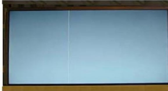
Vertical Line Source TAB IC Defect
