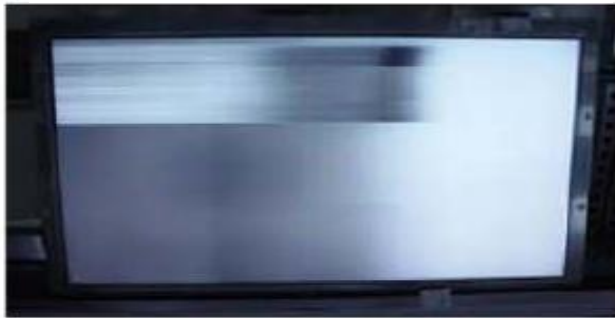
Horizontal Block Gate TAB IC Defect
