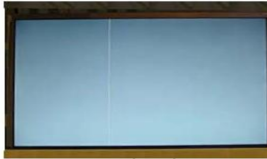
Vertical Line Source TAB IC Defect
