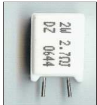
< Resistor, R101 > If R101 open state, it is change new component.
