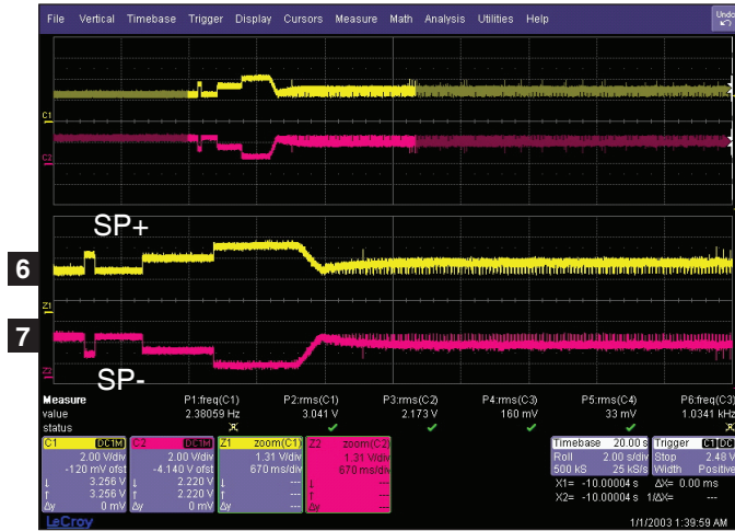
Figure 2-1. SP- & SP+ for driving SPINDLE motor (IC408 Pin17, 18)
