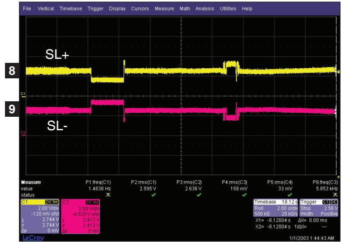
Figure 2-2. SL- & SL+ for driving SPINDLE motor (IC408 Pin11, 12)
