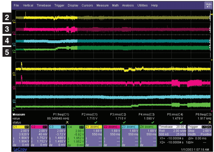
Figure 1-2. SERVO-FE, TE, FOD, RF (IC407 Pin61, 62, 63 / IC408 Pin1)
