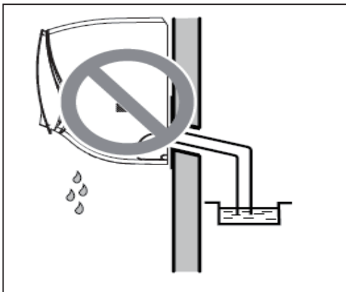
Case 5 : The end of the drain hose is locked into the water.
