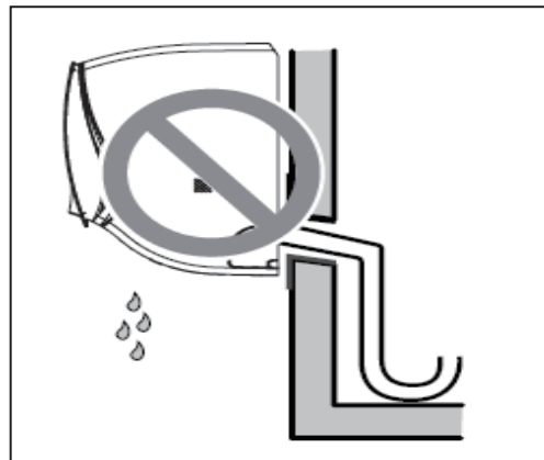
Case 6 : The end of drain hose is curled up.
