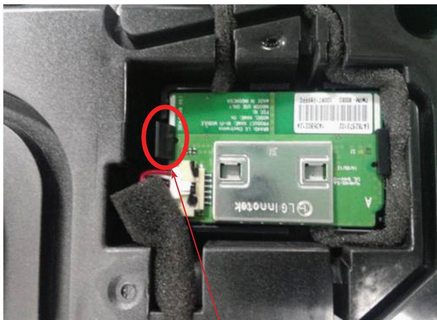
After Push the Guide hook, pull out Wi-Fi Module
