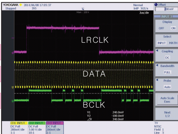
MICOM to AMP I2S IC700 PIN 23, 24, 25
