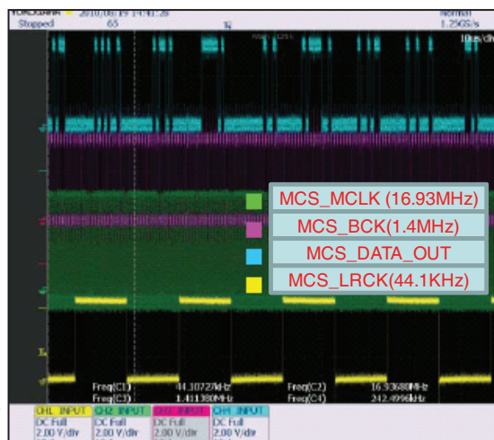
< Waveform of I2S audio interface signals >
