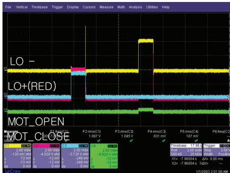
< Waveform for driving TRAY open/ close motor >
