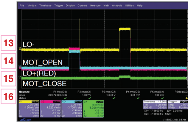
Fig 4-1. LO- & LO+ / MOT_OPEN & MOT_CLOSE for Driving TRAY Motor (IC400 pin6, 7, 9, 10)
