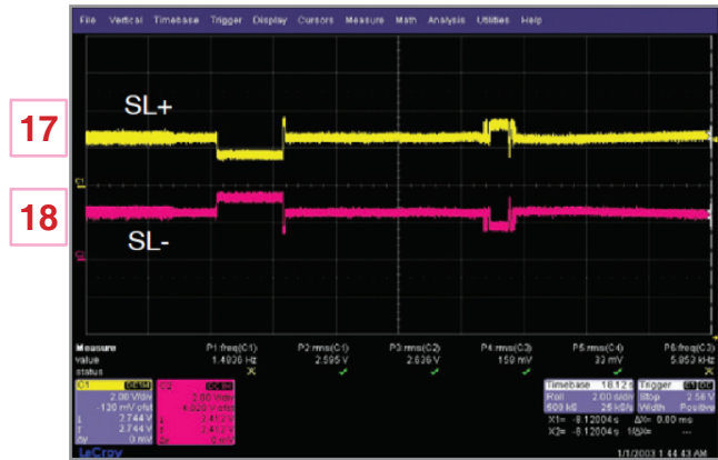
Fig 4-2. SL- & SL+ for Driving SPINDLE Motor (IC400 pin11, 12)
