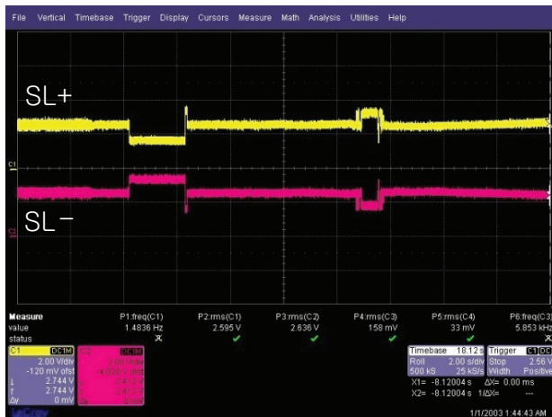
< Waveform of SLED- & SLED+ for driving SLED motor >
