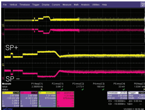
< Waveform of SP- & SP+ for driving SPINDLE motor >
