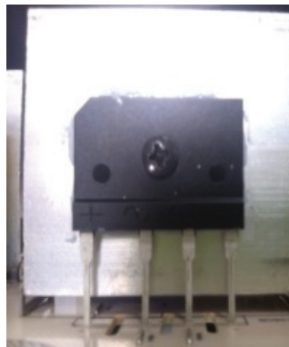
< BD901 > If BD901 is short-circuit, replace it with a new one.
