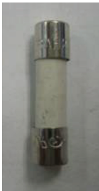
< F901 > If F901 is not short-circuit, replace it with a same specifications one.
