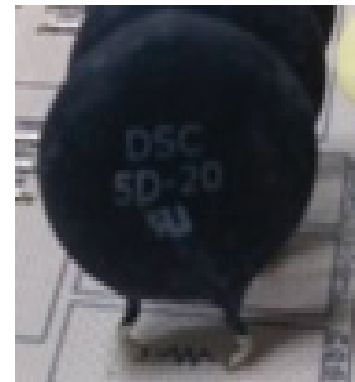
< TH900, TH901 > If TH900~TH901 is open, replace it with a new one.
