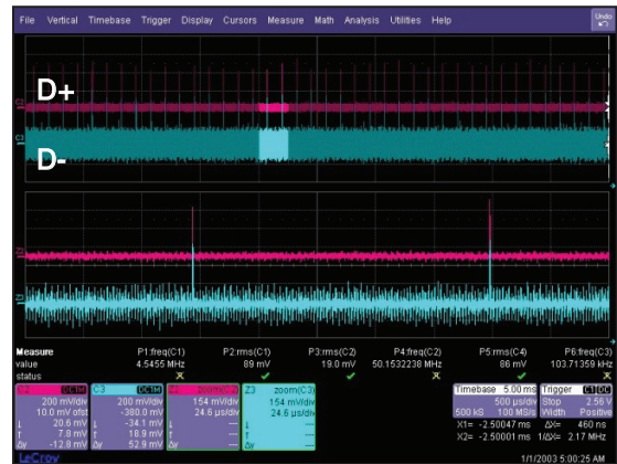
USB D+/D- (CN502 pin5, 6 & 8, 9) < Waveform of USB D± signal >
