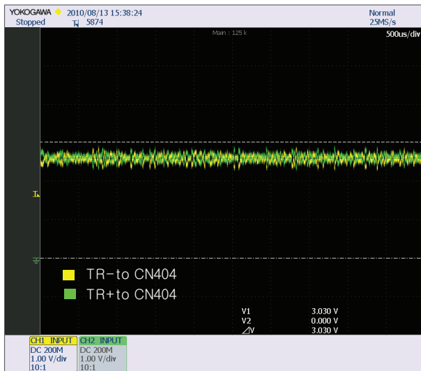
< Waveform of T± for driving TRACKING actuator >
