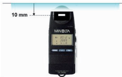
(Fig. 4-3-4) Measure brightness at 10mm inside the screen
