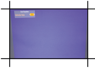
(Fig. 11-2-3) Example Before Auto Keystone Compensation
