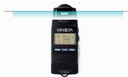
(Fig. 4-3-3) Measure brightness of screen boundary
