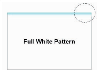
(Fig. 4-3-2) CL-200 for lighting margin inspection (right side)
