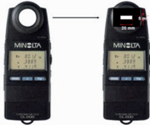
(Fig. 4-3-1) CL-200 for lighting margin inspection (right side)
