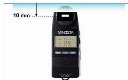
(Fig. 4-4-4) Measure brightness at 10mm inside the screen
