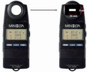
(Fig. 4-4-1) CL-200 for lighting margin inspection (right side)
