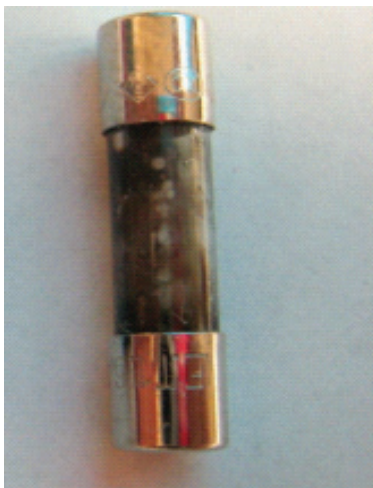
< Fuse, F901 > Can look at physical condition.
