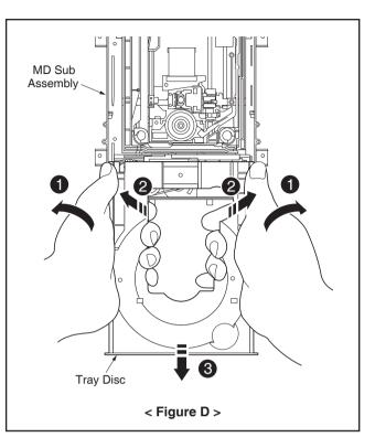
Grasp the both sides of the Tray Disc and lift it up as Figure D, and then pull the Tray Disc until it is separated from the MD Sub Assembly completely.
