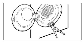
⑤ Open the door.⑥ Disassemble the clamp assembly.
