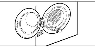
③ Put a flat ( - ) screwdriver into the openng of the hinge, and pull out the hinge cover.
