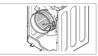
(i) Disassemble the clamp assembly.(i) Disassemble the Gasket.
