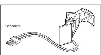
③ Disconnect the connector from PWB Harness.
