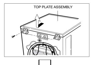
① Unscrew 2 screws on the back of the top plate.② Pull the top plate backward and upward as shown.
